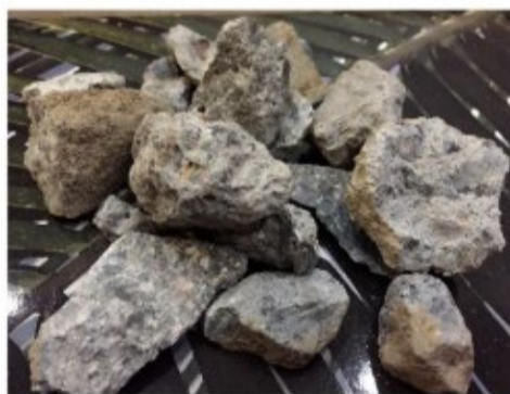
20-mm Recycled Aggregate
