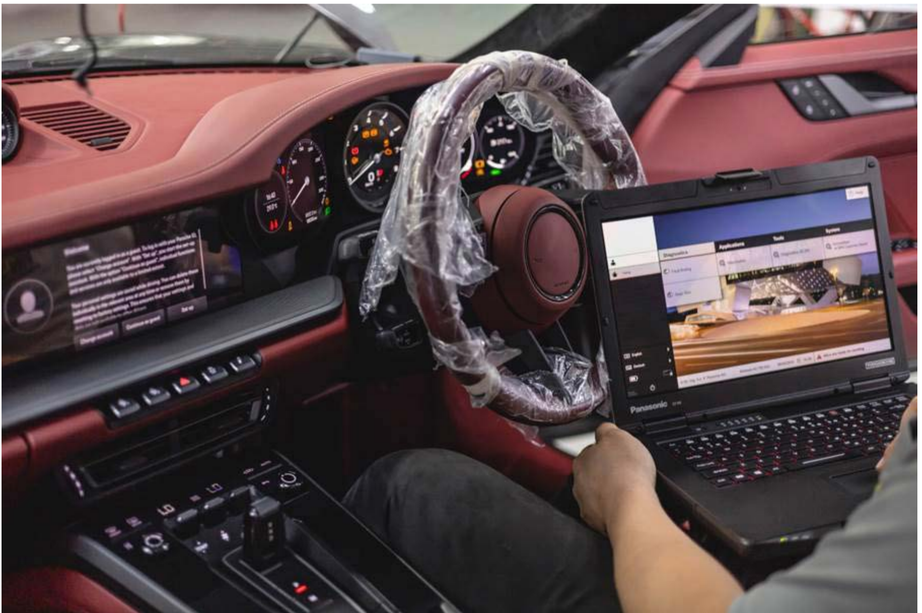
Diagnostics computer plugged in to check for issues
